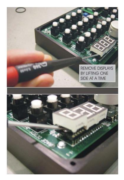
Pry up to release the display from the socket. Repeat for the other side. (It may be helpful to use your free hand to also pull up on the display to aide in removal, especially on the harder to access MAIN Level displays.)
