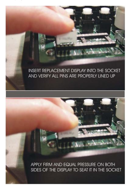
3) Repeat this for the five remaining displays. Note that there will be one unused socket position following the least significant digit at both the MAIN and HEADPHONE display positions.
