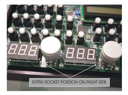
4) Finally, do a visual inspection of the displays to confirm that they properly aligned horizontally. If any of the display alignments are skewed, apply pressure to the side with your hand. This will bend the leads slightly and allow you to align the display.
