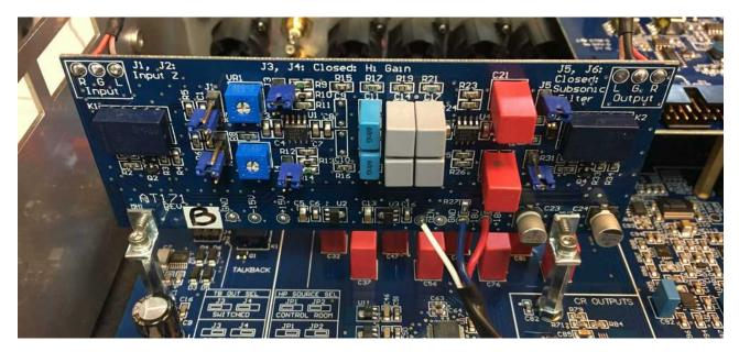
Grace Design 4689 Ute Highway, Longmont, CO 80503 tel: 303.823.8100 • fax: 303.823.8101 • email: service@gracedesign.com • <u>www.gracedesign.com</u> Page 3 of 6 6. Solder the red power wire to TP23 +18V on the m905 main board near the power supply connector. Solder the blue power wire to TP24 -18V. Solder the white control wire to P6 which is near the main processor U31.
