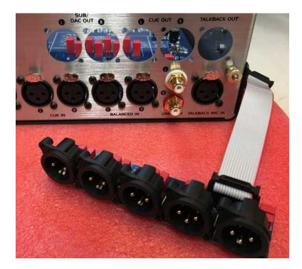
3. Unsolder the RCA input wires from the connectors and the main board. Wick up the solder to clean the PCB holes and connectors. Clean flux with alcohol and cotton swabs. Discard the wires.
