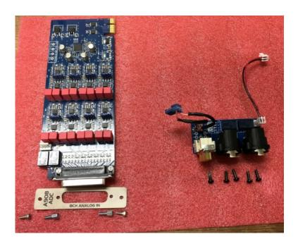
4. Install the stereo input PCBA with 5x H484 T8 Torx screws.
