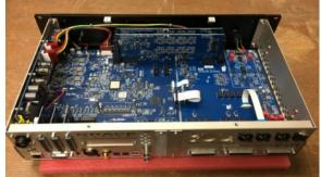
2. Remove the stereo inputs cover plate and ADC option cover plate(s). The stereo input cover plate is held on by two 3/32" Allen screws and two 1/4" Nyloc nuts. The ADC cover plates are held on by two 3/32" Allen screws. Retain these screws for the ADC installation.
