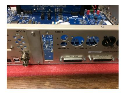
3. Prepare the ADC and stereo input PCBA. The ADC plate must be off for installation.
