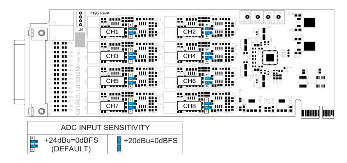
6. Install the ADC by inserting it from the inside of the unit and tilting the DB25 input connector down first, then aligning the card edge connector (PCI-E slot). When aligned, press down on the back of the ADC card to seat the connector. Repeat for the second ADC if installing.
