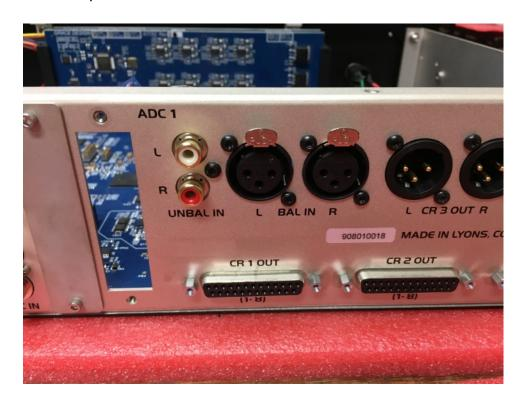
5. Set the ADC jumpers for your required sensitivity before installing the ADC. The default position is +24dBu = 0dBFS.
