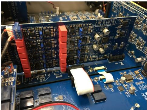
7. Install the ADC cover plate with the two H035 3/32" Allen screws that were previously removed and two H165 3/16" hex standoffs. The H165s will have Loctite pre-applied.
