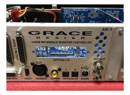
Connect the WA191 ribbon cable to J8 in the Aux I/O section of the m908 digital board.
