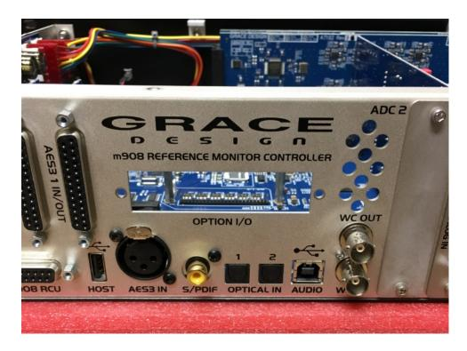
3. Connect the WA191 ribbon cable to J8 in the Aux I/O section of the m908 digital board.
