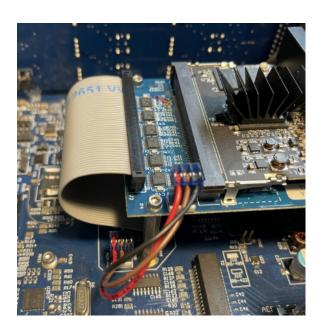
5. Re-install the top cover. Place the serial # label under the option card on the back. This concludes the m908 Ravenna option installation.
