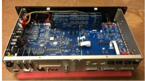
2. Remove the option slot cover plate. There are 2x 3/32" Allen head screws. Retain these screws for the option card install.
