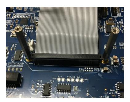
4. Place the AT188 Ravenna option card on the standoffs and through the option slot. Secure it with the two 3/32" Allen screws that were previously removed to the chassis. Use the included two 3/32" Allen screws with spring lock washers to secure it to the standoffs. Connect the 3 position jumper wire to J48 in the Aux I/O section of the m908 digital board.
